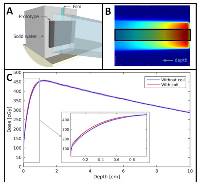
Figure 2. (a) Experimental setup for obtaining depth-dose information. A  $10 \times 10$  cm  $2$  beam from  $90^\circ$  was repeated with and without prototype. (b) The resulting films were converted to depth-dose curves by averaging 200 lines. (c) Depth-dose curves with and without prototype.
