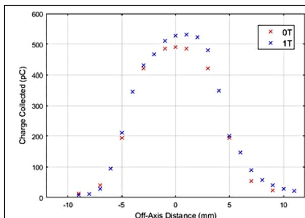
Fig 1: Profile at 1.5cm depth in solid water phantom with and without perpendicular 1T magnetic field for a  $0.9 \times 0.9 \text{cm}^2$  field
