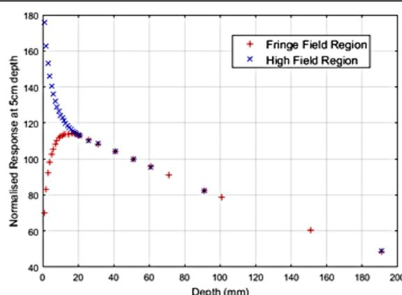
Fig 2: PDDs at different magnetic field strengths, taken in a  $30 \times 30 \times 30 \text{cm}^3$  solid water phantom on the Australian MRI-linac
