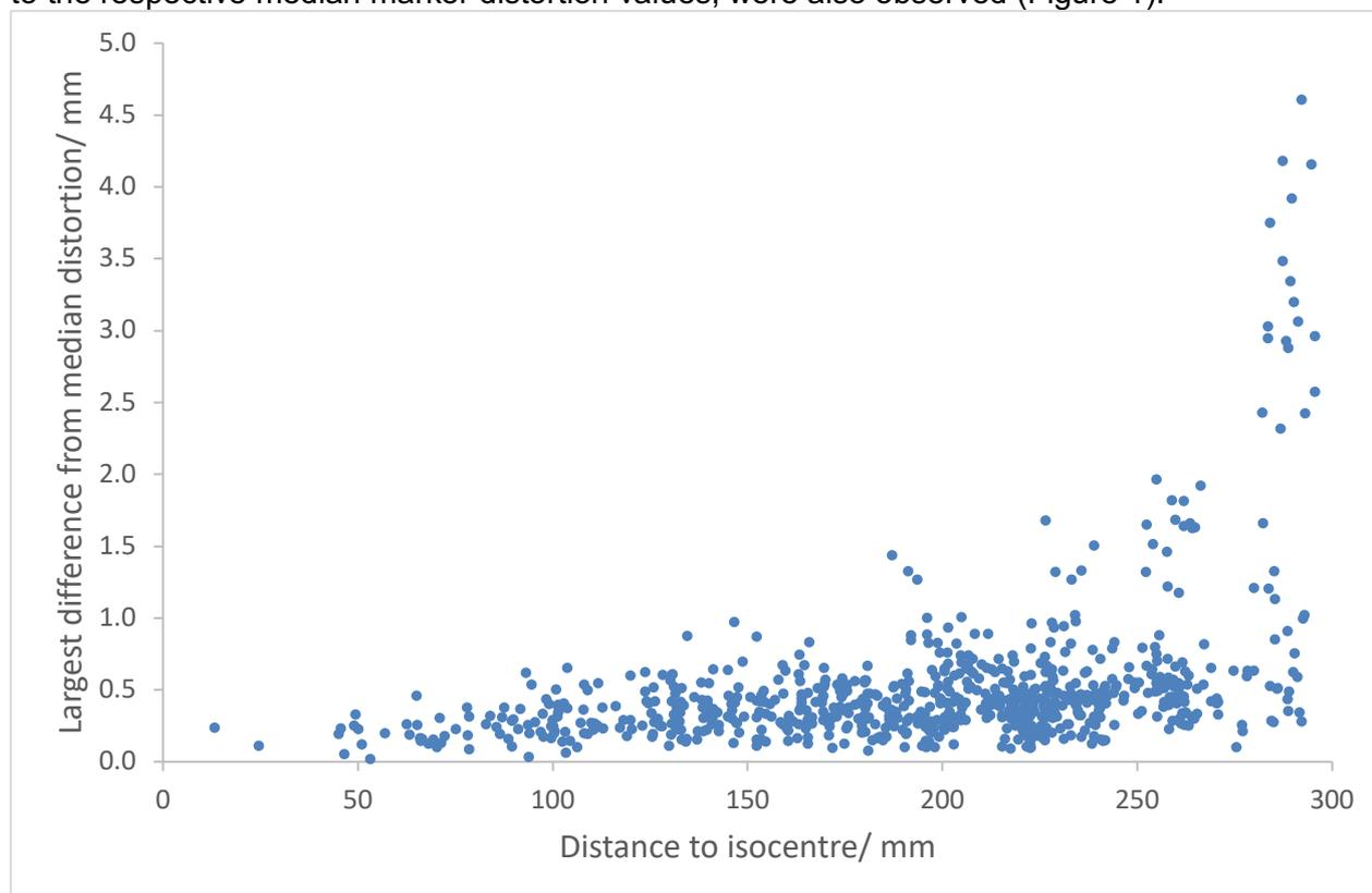
Figure 1. Showing the maximum deviation of marker distortions from their respective median distortion values over the measurement period for the Siemens Aera 3D sequence, as an example. The results are shown as a function of the radial distance to isocentre.
